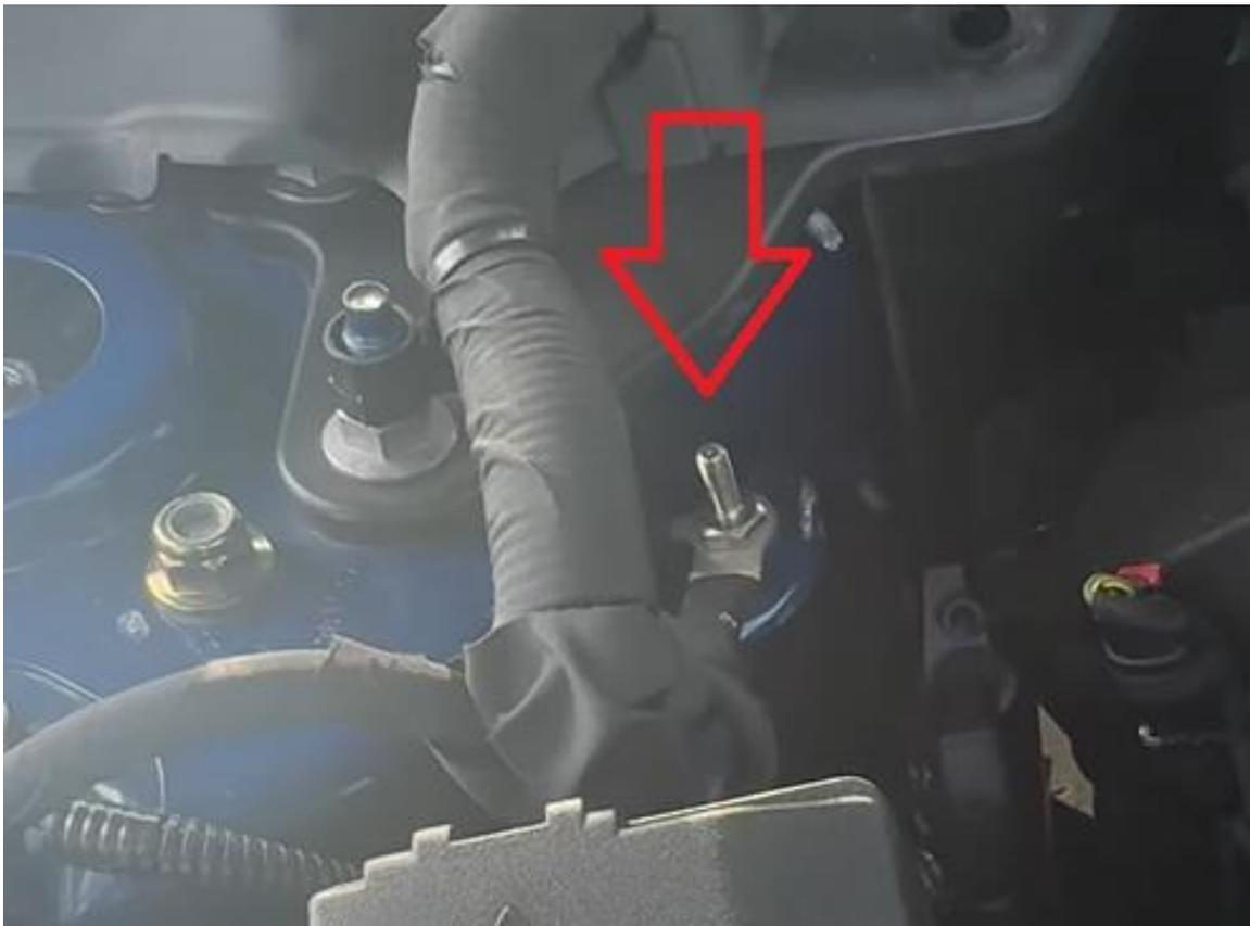
Install J&L can onto J&L bracket using the two supplied screws, the J&L Logo's should match the same direction.
